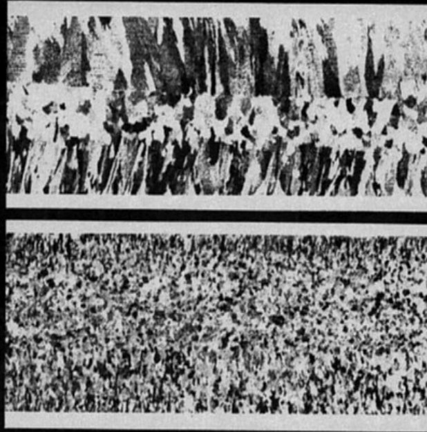
Fig. 2-5. Effect of addition of a grain refiner on the cast grain size and shape of commercially pure aluminum (1100 aluminum) cast by a two-belt method. Both pictures are of longitudinal sections, shown at actual size. The upper slab was cast without a grain refiner and the lower with a grain refiner addition (e.g., titanium or titanium and boron). (From Metals Handbook, 8th Ed., Vol 8, American Society for Metals, Metals Park, Ohio, 1973)
